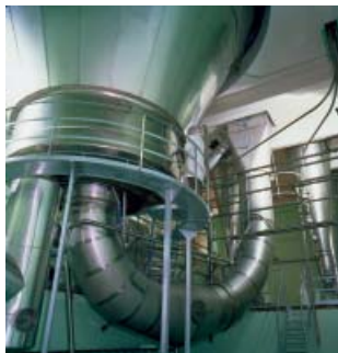
2 Stage Conical Spray Dryer
